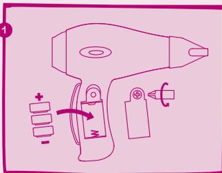
(EN): To replace batteries: Unscrew the battery cover and replace 3 x AG13 (1.5V) size batteries.
